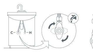
Turn off the water supply valve and then disconnect the 3/8" female compression end of the supply line attached to the faucet.
