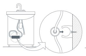
Secure Mounting bracket in a convenient location.
