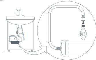
Connect the 3/8" female compression end of the inlet hose to the water supply valve. Inlet is on the cap side.
