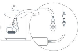
Connect the 3/8" male compression end of the outlet hose to the end of the supply line attached to the faucet.
