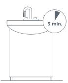
Activate the filter by allowing the water to flow for 3 minutes.
