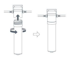
Screw in the new Woder Filter cartridge. The water cuts back on when you screw the new filter on.
