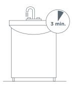
Activate the filter by allowing the water to flow for 3 minutes.
