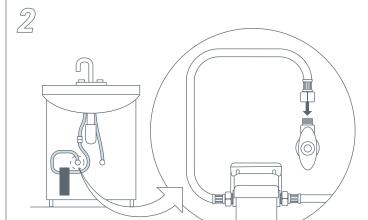
Connect the 3/8" female compression end of the inlet hose to the water supply valve.
