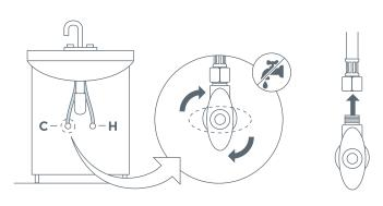
Turn off the water supply valve and then disconnect the 3/8" female compression end of the supply line attached to the faucet.
